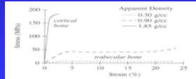
Figure 3. Examples of typical compressive stress-strain behaviors of trabecular and cortical bone for different apparent densities. (Reproduced with permission from Manuwy SM, Hayes WC. Mechanical Properties of Cortical and Trabecular Bone . In: Hall DC (ed): Bone . Boca Raton, FL: CRC Press, 1993, vol 2, pp 290-303.)
