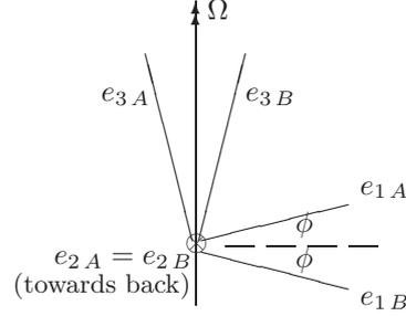
Fig. 1. Two rigid bodies in a situation from which (4),(6) do not synchronize attitudes for small  $\sigma$ . All vectors lie in the same plane, except  $e_{2A} = e_{2B}$  perpendicular to the page.
