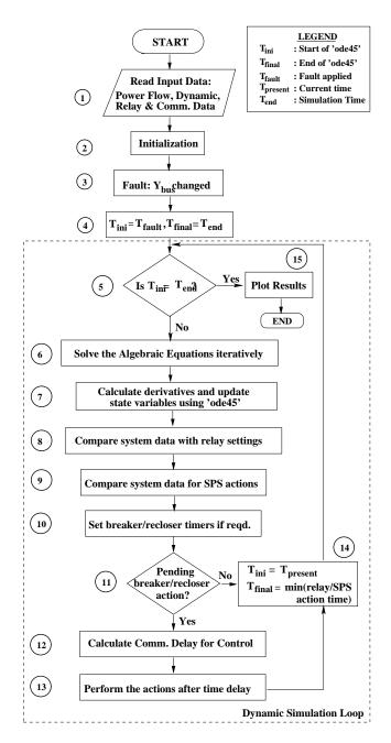
Figure 1: Flow Chart of the Dynamic Simulation Program
