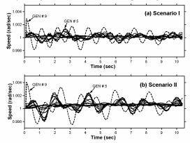
Figure 3: Speed rotor deviations following a short circuit at bus 28. a) Scenario I, b) Scenario II.
