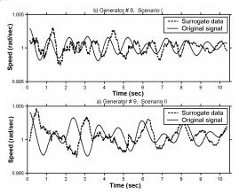
Figure 7: Comparison between original signal and the surrogate data for scenarios I and II. Generator #9.
