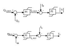
Fig. 6- Dual Static Converter Connected to the Stator of the Generator – Active and Reactive Powers Control
