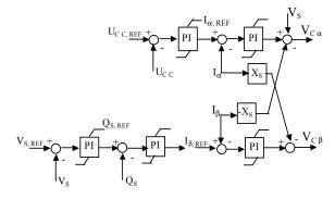
Fig. 8 -Control Loops for the Converter Connected to the Electrical
