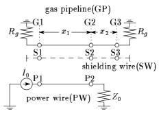
Figure 1: A system composed of an overhead line and a buried gas pipeline
