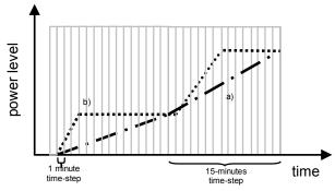
Figure 1 Examples of power profiles within 15-minutes periods: a) linear profile, b) maximum allowed ramp followed by constant level.
