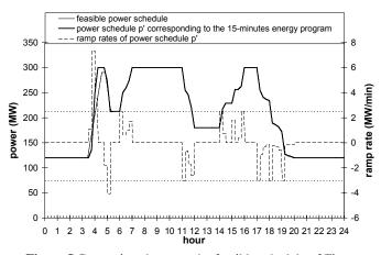
**Figure 5** Comparison between the feasible schedule of Figure 2 and the power schedule  $\mathbf{p}'$ , solution of the second problem (for  $w_1'=1$ ,  $w_2'=10^3$ ,  $w_3'=1$ ), with its ramp rates.
