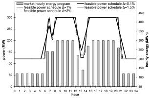
**Figure 8** Comparison between the feasible schedules obtained for different values of the ramp rate limit  $\Delta = \Delta_u = \Delta_d$ : 0.5%, 1%, 1.5% and 2% of  $P_{max}$ . Results obtained for two market hourly energy programs: a) profile 1, b) Profile 2.  $(w_I=1, w_2=1)$
