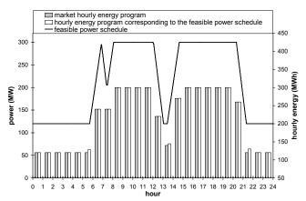
**Figure 6** Feasible power level profile of a thermoelectric unit (whose data are shown in Table 1) and the hourly energies corresponding to the power schedules, obtained from a given market hourly energy program (for  $w_l$ =1 and  $w_2$ =1).
