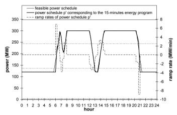
**Figure 7** Comparison between the feasible schedule of Figure 6 and the power schedule  $\mathbf{p}'$ , solution of the second problem (for  $w_I'=1$ ,  $w_2'=10^3$ ,  $w_3'=1$ ), with its ramp rates.
