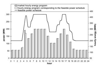
**Figure 2** Example of a feasible power level profile of a thermoelectric unit (whose data are shown in Table 1) and the hourly energies corresponding to the power schedules, obtained from a given market hourly energy program (for  $w_1$ =1 and  $w_2$ =1).
