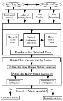
Figure 1: Architecture of BCU-DSA System
