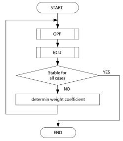
Figure 10: OPF algorithm considering dynamic stability
