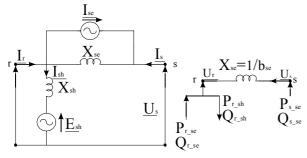
**Figure 3:** Shunt and series sides of the UPFC converted into two power injections at buses r and s.
