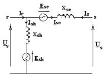
Figure 2: UPFC equivalent circuit
