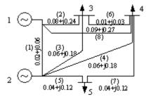
**Figure 5:** Test power system (1 to 5: buses, (1) to (8): lines) Base power 100 MVA, base voltage 150kV
