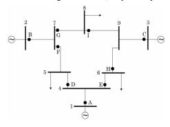
Figure 4: Anderson & Fouad 3-machine 9-bus system.
