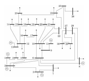
Figure 5: IEEE 6-machine 30-bus system
