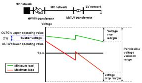
Figure 2: Available voltage rise and drop margins.
