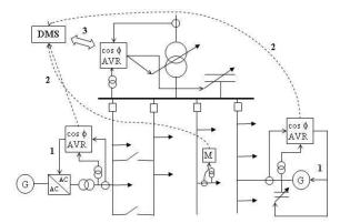
Figure 1: Concept for voltage level management.
