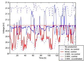
Figure 3: Voltages of wind turbine connection point.
