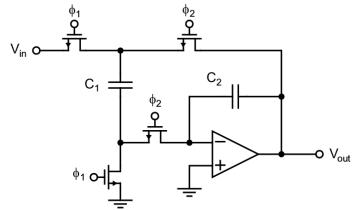
$${}^{3}H(z) = rac{z^{-1}}{1+C_2/C_1(1-z^{-1})}, \ f_{-3dB} = rac{1}{2\pi}rac{C_1}{C_2}f_s$$
