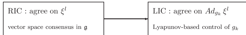
Figure 3: Total coordination as consensus on left-invariant velocity and Lyapunov-based control to left-invariant coordination.
