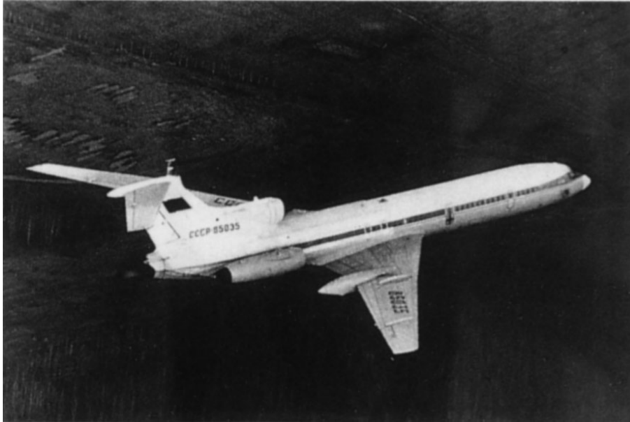
Tupolev 155 (1988), one engine on H_2
