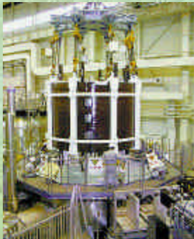
REMOTE MAINTENANCE OF DIVERTOR CASSETTE
